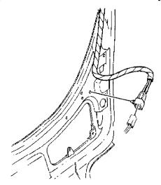
3. Disconnect the high mount stop lamp connector from the electrical harness.
