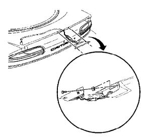
1. Position the high mount stop lamp to the rear end spoiler.
