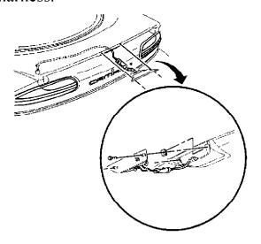
4. Remove the high mount stop lamp from the rear end spoiler.
